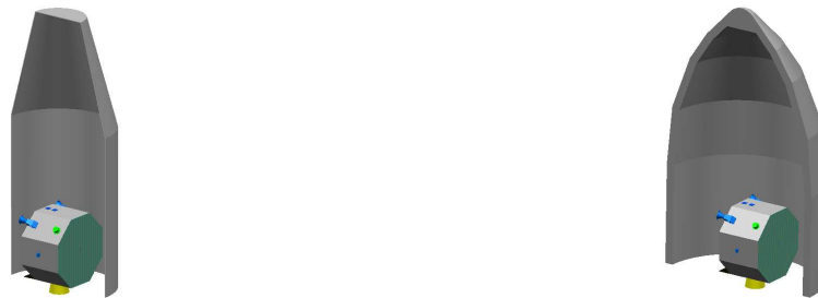
Figure 12: BIOSAT accommodation in the Athena 1 launch fairing (left) and the DNEPR launch fairing (right).
