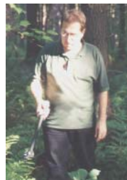
Figures 1.1 TRAC measures light under the canopy while the operator holds it levelled and walks at a constant slow pace.
