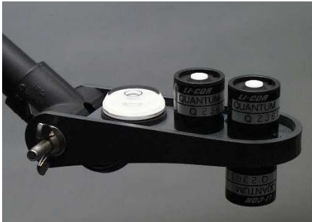
Figure 2.1: TRAC consists of 3 PAR sensors (400 to 700 nm) and amplifiers, an analog-to-digital converter, a microprocessor, a battery backed memory, a clock and serial I/O circuitry. A power switch controls the power to all components of the system except the memory. A control button controls the operating mode when the power is on. This button is also used to insert distance/time markers.
